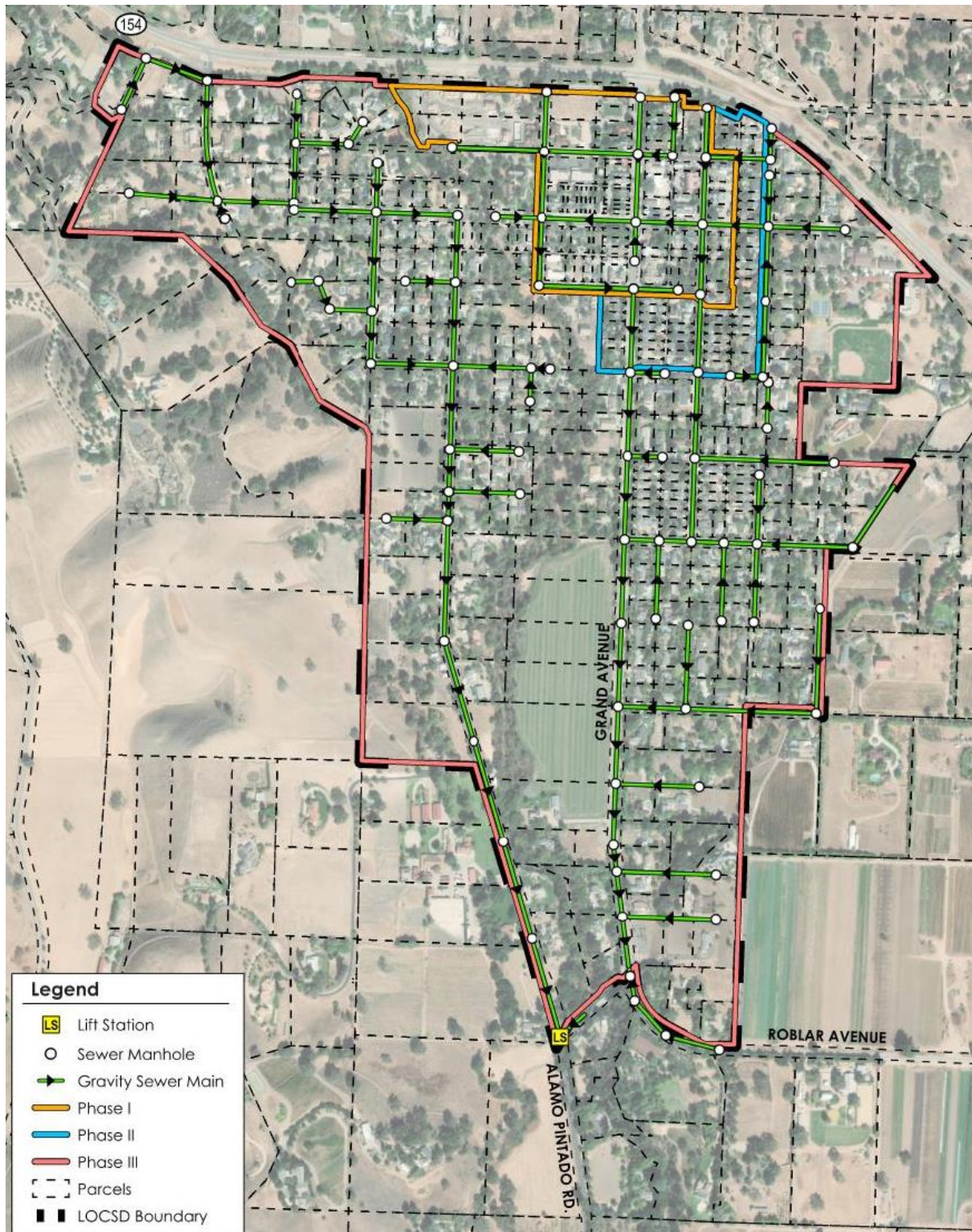
Figure 1: Los Olivos Preliminary Gravity Sewer Collection Layout
